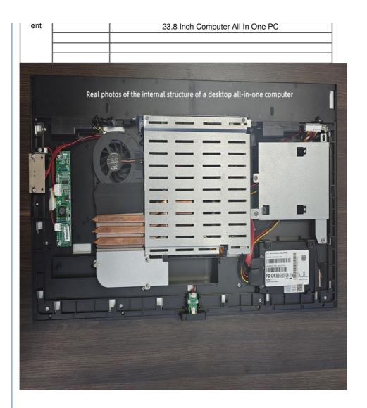
Internal structure diagram of desktop all-in-one computer
